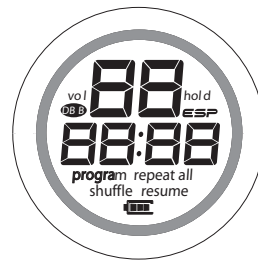
test pattern 2 (alternate segments activated)
