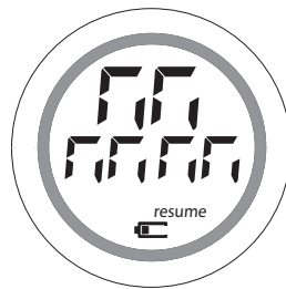
test pattern 2 (alternate segments activated)
